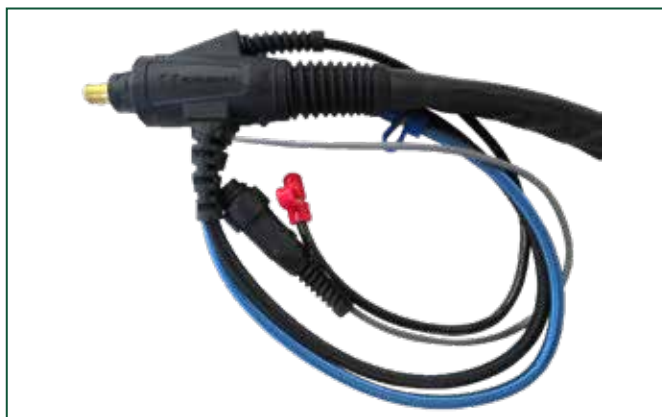
Cable connector for water-cooled TIG 321/401/451 welding torch.
