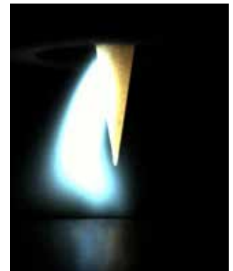
Low-quality tungsten: typically sideways arc ignition, the arc flashes and wanders slowly to the electrode tip which has to be cut off and reground.
