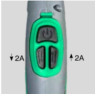
Up/Down module with 3-function key for adjustment of welding current. The welding current is increased / reduced with 2 amps. Long press for constant increase / decrease. Art. no. ....80300064* * Applies to software versions as of 2.17
