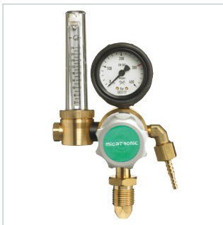
ARGON/MIX OPTIMATOR 1 FLOWMETER BOTTOM CONNECTION Argon/mix Optimator with built-in gas saver. Gas consumption can be reduced by up to 50%. Result = fewer replacements of gas cylinders and improved production efficiency. Inlet thread: G5/8"ext Outlet thread: G3/8" Art. no. ....81963080
