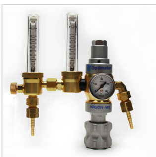
ARGON/MIX OPTIMATOR 2 FLOWMETRES Argon/mix Optimator with 2 flowmetres. Used for shielding gas and back-up gas from the same gas cylinder. Equipped with gas saver. Gas consumption can be reduced by up to 50%. Inlet thread: W21,8x14/1" Outlet thread: G1/4" Art. no. ....81963050
