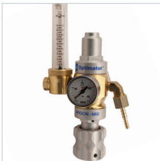
ARGON/MIX OPTIMATOR 1 FLOWMETER Argon/mix Optimator with built-in gas saver. Gas consumption can be reduced by up to 50%. Result = fewer replacements of gas cylinders and improved production efficiency. Inlet thread: W21,8x14/1" Outlet thread: G3/8" Art. no. ....81963309
