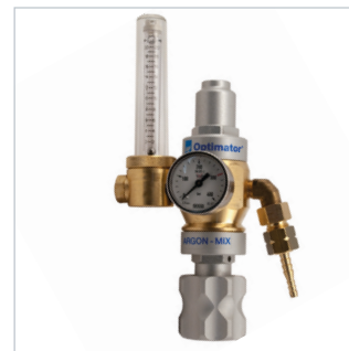
ARGON/MIX OPTIMATOR 1 FLOWMETER BOTTOM CONNECTION Argon/mix Optimator with built-in gas saver. Gas consumption can be reduced by up to 50%. Result = fewer replacements of gas cylinders and improved production efficiency. Inlet thread: G5/8"ext Outlet thread: G3/8" Art. no. ....81963080
