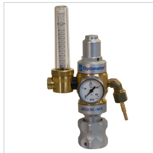
ARGON/MIX OPTIMATOR 1 FLOWMETER Argon/mix Optimator with built-in gas saver. Gas consumption can be reduced by up to 50%. Result = fewer replacements of gas cylinders and improved production efficiency. Inlet thread: W21,8x14/1" Outlet thread: G1/4" Art. no. ....81963047
