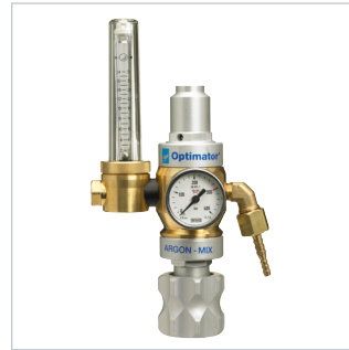
ARGON/MIX OPTIMATOR 1 FLOWMETER Argon/mix Optimator with built-in gas saver. Gas consumption can be reduced by up to 50%. Result = fewer replacements of gas cylinders and improved production efficiency. Inlet thread: W24.32x14/1" Outlet thread: G3/8" Art. no. ....81963041
