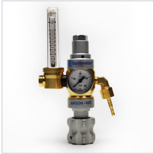
ARGON/MIX OPTIMATOR 1 FLOWMETER Argon/mix Optimator with built-in gas saver. Gas consumption can be reduced by up to 50%. Result = fewer replacements of gas cylinders and improved production efficiency. Inlet thread: W24.32x14/1" Outlet thread: G3/8" Art. no. ....81963041
