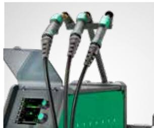
Control unit for adjustment of welding current at the torch handle (item number 80100402)
