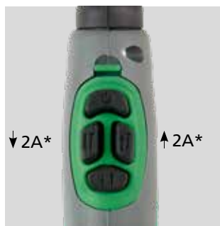
Up/Down module with 4-function key for adjustment of welding current incl. TIG-A Tack function. The welding current is increased / reduced with 2 amps. Long press for constant increase / decrease. 80300063
