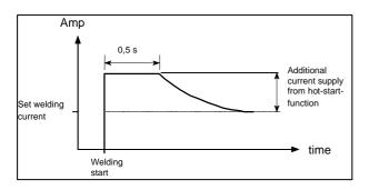
The hot start value reflects the percentage value by which initial current is increased, and can be set between 0% and 100%.
