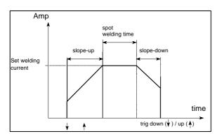
If spot time is changed during welding, this change will not be carried into effect until next welding process.
