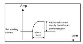
Arc power can be adjusted between 0 and 150% of the welding current setting.
