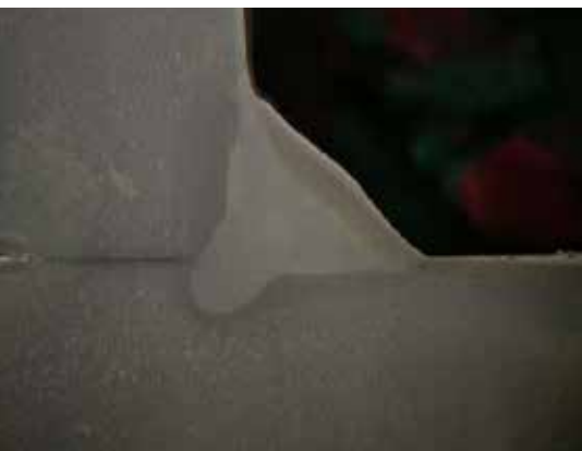
PowerArc™ ensures full penetration in fillet welds and butt welds and increased welding speed using mild and stainless steels.
