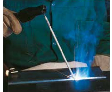
MMA in a V-joint
