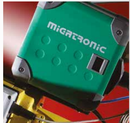
RWF - Robot Wire Feeder.
