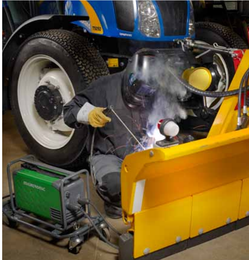
The handy Delta with protective frame and trolley with wheels is here used for repair of a snow shovel using basic electrodes.
