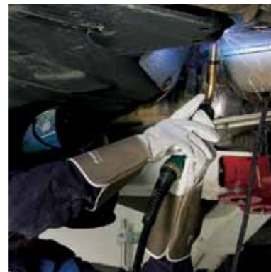
Trim of welding parameters using the Dialog torch
